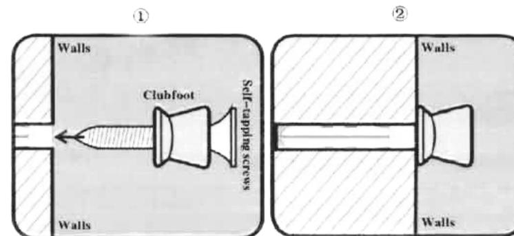
4. Fix 4 feet to the clubfeet, screw up the feet with a wrench until totally fixed.
