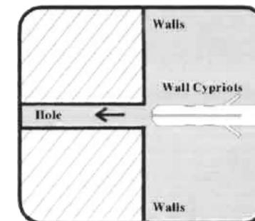
3. Put the self-tapping screws through the center hole of the clubfoot and fix it to the wall.
